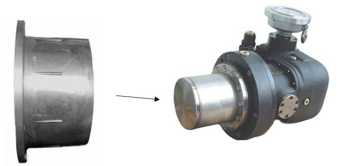
1. Slide the outer magnet onto the motor shaft, making sure the key is in place. The end of the pump shaft should then be flush with the magnet hub.
