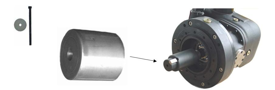
1. Slide the inner magnet over the intermediate shaft, making sure key is in place.
