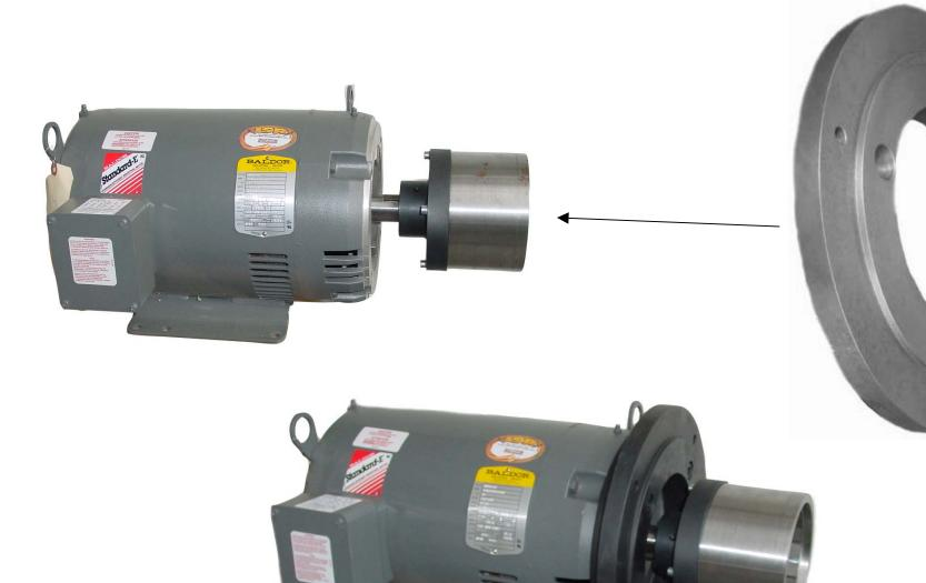
1. Align the 2 assemblies and carefully bring them together. Make sure fingers are not between the bellhousing and motor flange.
