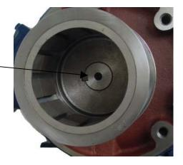
1. Place motor flange on the motor. Only socket head screws can be used to tighten in place.
